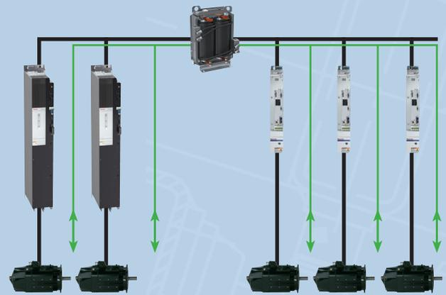
motors operate in generator and motor modes
