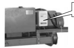
Mounted receiver in a firmed site where the dual color LED can be seen
